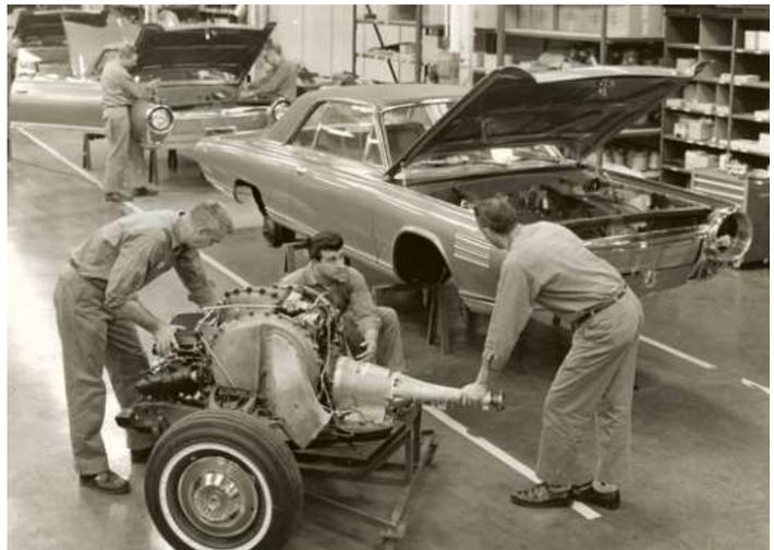
■ Chrysler employees installing a turbine drivetrain in a Ghia body. These cars used a coil spring front suspension instead of Chrysler's usual torsion bars; this was needed to accommodate the turbine's girth.
