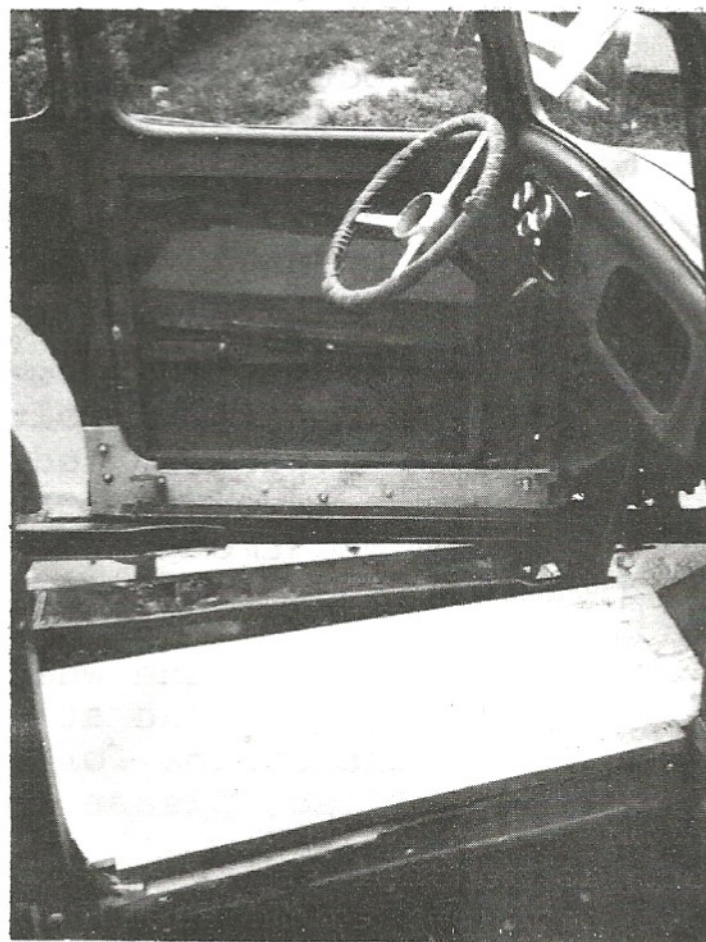
New flooring using original trans- mission tunnel note ash side- members.
