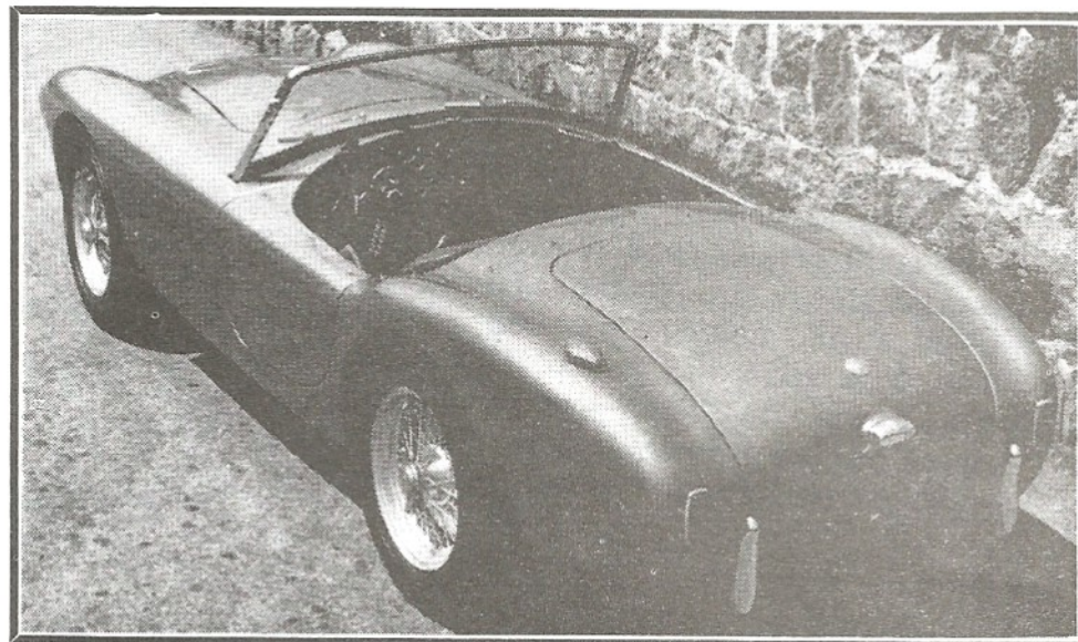
AC Ace, a 1953 car that had a tubular chassis and all-independent suspension, had wonderfully pure modern roadster styling.
