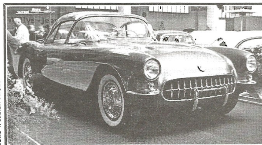
1957 Corvette was a high point with its fuel injection, all-synchro 4-speed gearbox and good-looking removable hardtop.
