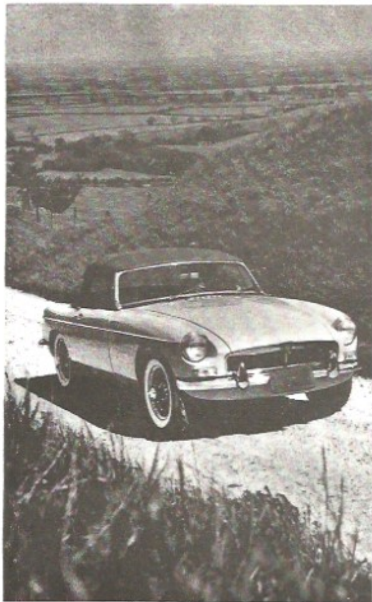
Removable hardtop will be available soon. Dished floor would allow inversion of spare, increasing luggage space.
